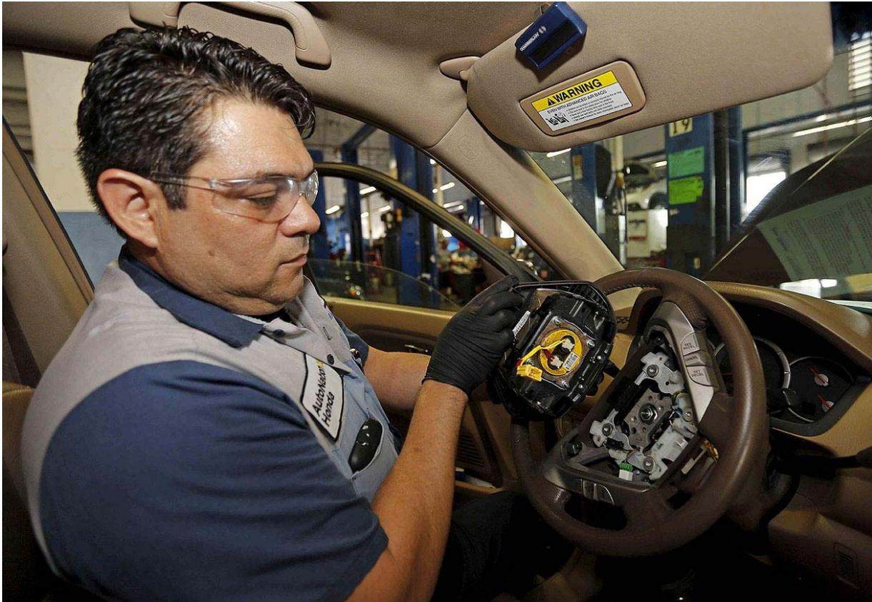
Technician Edward Bonilla with a recalled Takata airbag inflator after it was removed from a Honda Pilot at the AutoNation Honda dealership in Miami, Fla., in June 2015. Honda, which has been Takata's largest customer, has replaced about 5.4 million inflators -- more than half of those it had recalled through December.
